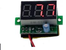
Connect the voltage display (if required) to the terminal marked "MON" on the circuit board.
